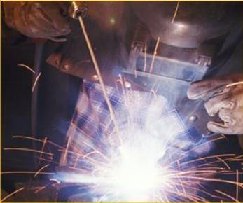
The U.S. Chemical Safety & Hazard Investigation Board has identified more than 60 fatalities since 1990 due to explosions and fires from hot work activities on tanks. Hot work is defined as “work involving burning, grinding, welding, gouging or a similar operation that is capable of initiating fires or explosions.”
